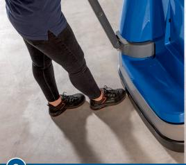
Vehicle equipped with foot protection switch. Collision with foot detected. Vehicle stops.
