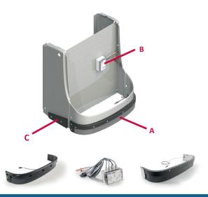
**Area Sensor [A]** The Area sensor provides the controller with a signal which changes when actuated (application of pressure). The deflector plate and the sensor are available in a smart spare part concept. These components can be easily replaced without disassembling the total area sensor.
