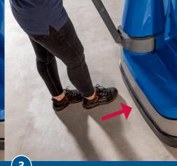
Vehicle equipped with foot protection switch. After collision and stop, the vehicle reverses. 3
