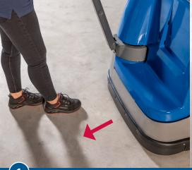
Vehicle equipped with foot protection switch. No collision with the foot.
