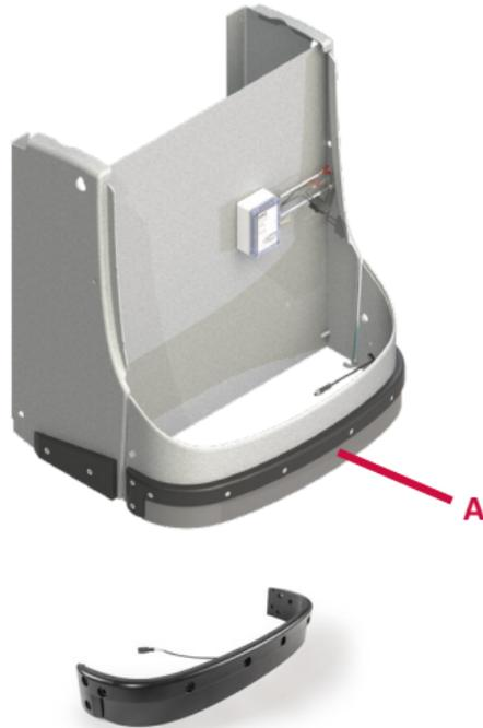
**Area Sensor [A]** The Area sensor provides the controller with a signal which changes when actuated (application of pressure). The deflector plate and the sensor are available in a smart spare part concept. These components can be easily replaced without disassembling the total area sensor.
